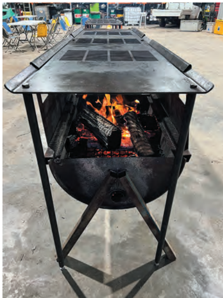
The BBQ designer added heat skirts to reflect some of the heat so people could get closer to the hotplate and talk a lot longer.
